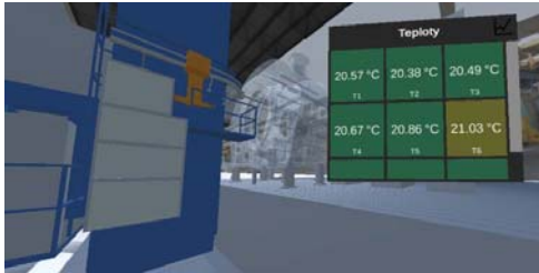
Fig. 4. Temperature display on the digital twin
