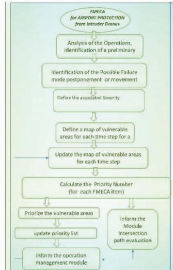
Fig. 3. This sketch shows the FMECA methodology.
