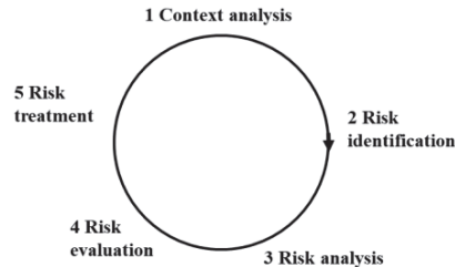
Fig. 1. Risk cycle process: 5-step risk analysis and management process according to ISO 31000 (2018) clause 6.
