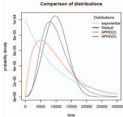
Fig. 5. Probability density functions of Weibull and exponential distributions with the same mean value. The Weibull distribution is approximated by two acyclic phase type distributions of order 2 and 5 accordingly.
