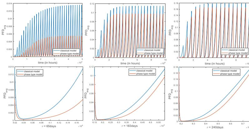
Fig. 7  $PFD_{avg}$  of an ESV for different inspection lengths:  $\tau = 2, 6$  and 8 months, shown in longer time perspective (top plate) and during one interval (bottom plate)
