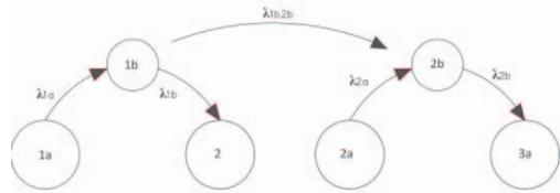
Fig. 2 Branching of two CTMCs resulting from APHD approximation of Weibull distributed transition times between main states of the "classical" Markov model. States 1a and 2a correspond to main degradation states 1 and 2 from the previous model. States 1b and 2b are artificial intermediate states added in the result of phase-type approximation.
