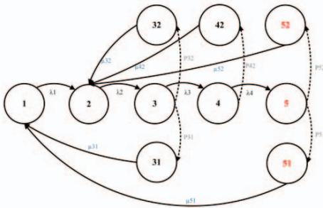
Fig. 1. Multiphase Markov model including maintenance. Dashed lines indicate repair decisions. Logical states are described by double digits, for instance in state 32, the first digit denotes that the physical degradation is at level 3, and the second digit says that the valve condition will be improved to state 2.
