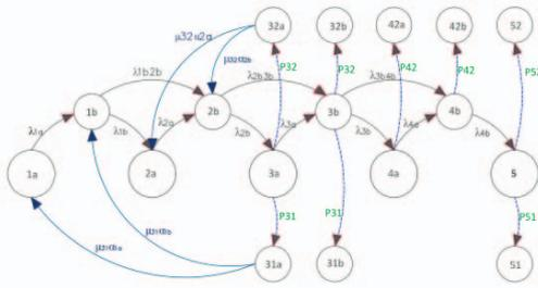
Fig.4 Phase-expanded degradation model including maintenance strategy.
