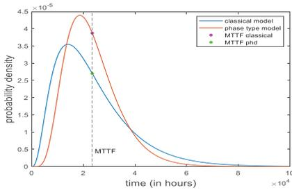
Fig. 6. Probability distributions of time to failure of an ESV, modelled by 5 state CTMC (classical model) and its phase expansion with 9states (phase type model).
