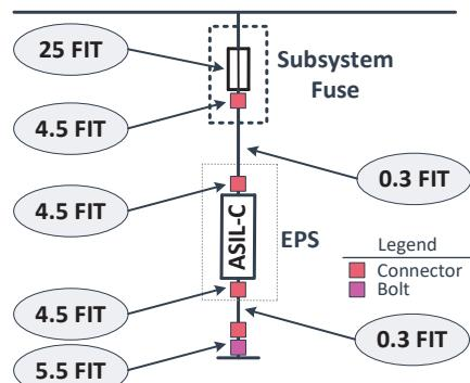
Fig. 9. Example failure rates of single channel connection
