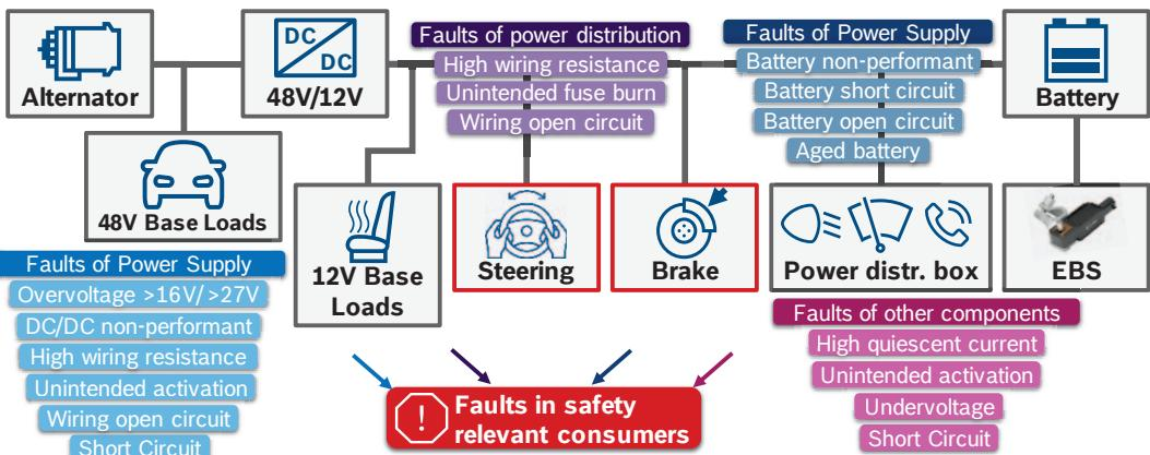
Fig. 3. Schematically powernet topology design
