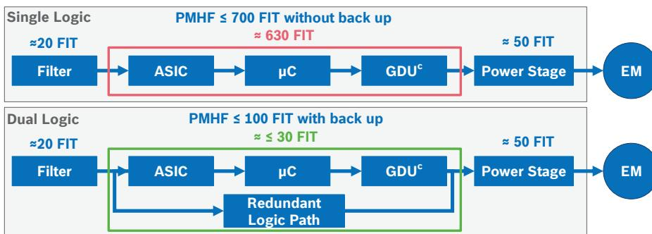
Fig. 8. EPS single logic- vs. dual logic system
