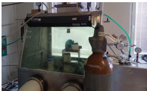
Fig.1. The experimental glove box with CLARE 4.0 electric furnace for molten salt static corrosion experiments.
