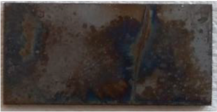
Fig.3. The picture of AISI 316L sample after the 30 days / 550 °C exposure to molten NaF-NaBF 4 salt.
