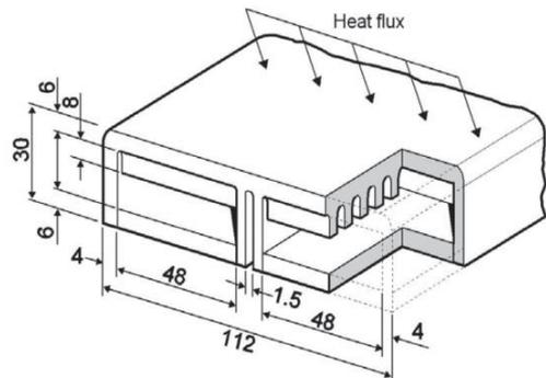
Fig. 2. Scheme of hypervapotron; processed according to (Pitonak 2016).
