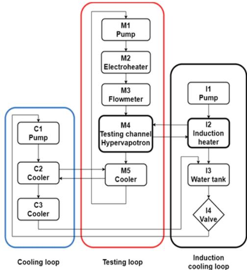
Fig. 4. A process model of an experiment that investigates the cooling process using a hypervapotron device (Gleitz 2022).
