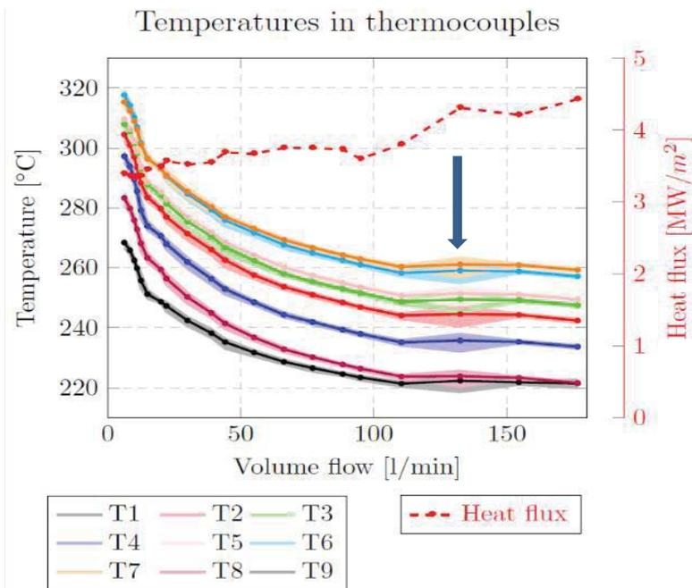
Fig. 5. The course of temperature decreases with flow (Gleit 2022).
