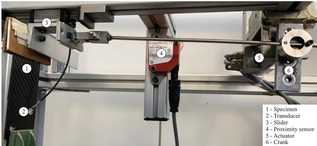
Fig. 2. Experimental set-up for cyclic loading
