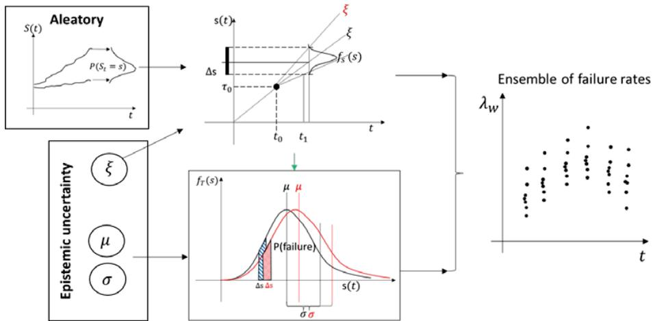
Fig. 1. Illustration of how uncertainty is propagated from input parameters to component failure rates.
