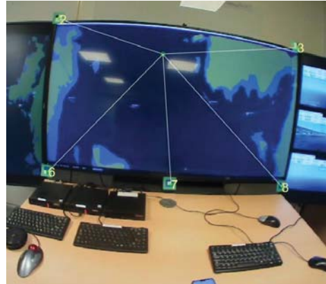
Fig 1. View from eye-tracking glasses and camera used by participants. Image recognition is used to identify markers and display information overlay.
