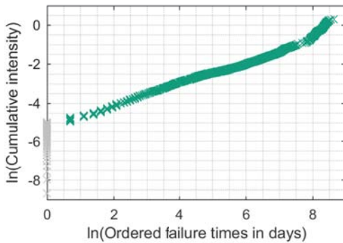
Fig. 4. Plot of natural logarithm of non-parametric cumulative failure intensities vs. logarithm of failure times for the evaluated data set (excluding zero-time failures in grey)
